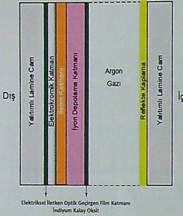
Şekil 12. Elektrokromik cam kesiti (Selkowitz ve Anders; 2008). Diag. 12. Electrochromic glass cross-section (Selkowitz and Anders; 2008).
